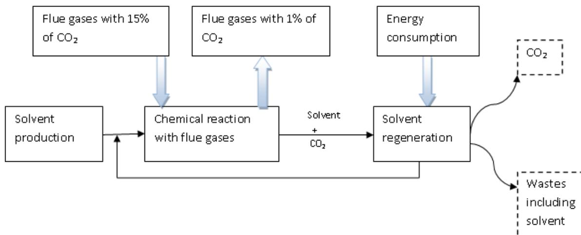
Positioned downstream, this capture process can be added to existing coal or gas power plants, blast furnaces, cement kilns or factories that emit large  $CO_2$  amounts.
